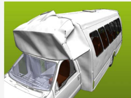
Figure 3. Deformation of the paratransit bus after the roadside accident (left), is very consistent with the deformation of the paratransit bus observed during F.E. analysis of the rollover performed following the requirements of the FDOT Standard (right).
