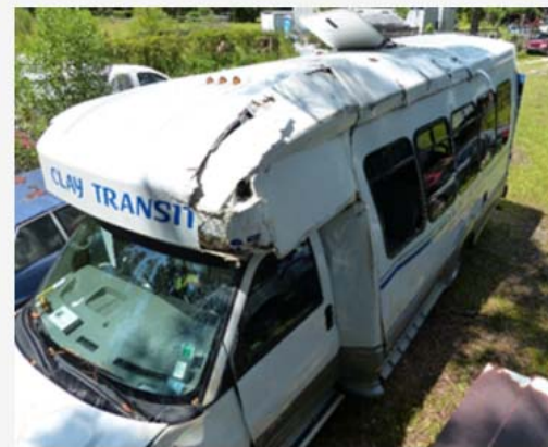
Figure 3. Deformation of the paratransit bus after the roadside accident (left), is very consistent with the deformation of the paratransit bus observed during F.E. analysis of the rollover performed following the requirements of the FDOT Standard (right).
