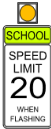
S5-1 Flashing Beacon
